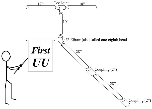
Banner poles should be constructed of plastic PVC pipe, available at hardware and plumbing supply stores.
